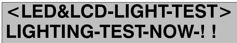
Figure 5-11. Control Panel Display Test Pattern
